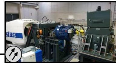
4 MW On-Shore Wind Turbine Test Bench
